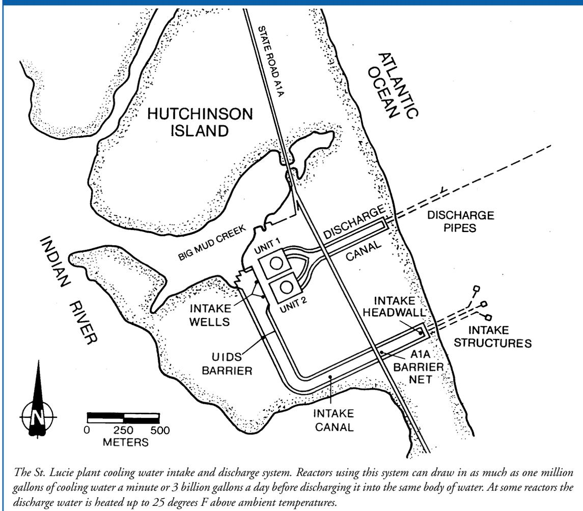
(*entrained*) into the plant's cooling canals through an intake canal or tunnel. Larger species, such as sea turtles and seals, have drowned or suffocated during entrainment. Others become impinged against trash rakes or net. Fish larvae, spawn, and fingerlings (young fish), are destroyed by their passage through the plant systems and, when discharged at the end of the cooling process, are described by the industry as "debris."
